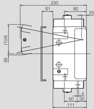
Arc space dimensions (S1) is 30 mm for 220 V of the circuit voltage, 60 mm for 600 V of the circuit voltage.
