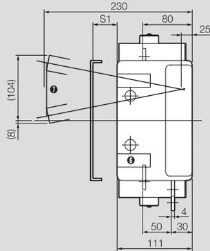
Arc space dimensions (S1) is 30 mm for 220 V of the circuit voltage, 60 mm for 600 V of the circuit voltage.
