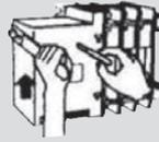
While the screwdriver is being pushed into the S section, control the manual handle in the direction indicated by the arrow.
